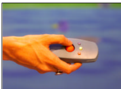
Figure 3: The wand - an interaction device for a VR environment
